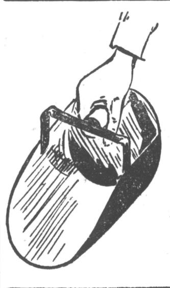
Here's a right smart idea for a feed and grain scoop that eliminates the wrist strain of scoops with the usual projecting handles. For a large scoop, one that can be used in sacking grain, 20-gauge galvanized material is about right. The scrap iron brace to which the front end of the handle is bolted helps hold light metal in shape.
